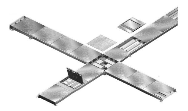
Flush Floor Trunking system is designed for the distribution of power, voice & data services on the screed floor. This system is widely used in commercial offices and in this system both Trunking & Floor Boxes are flushed to the screed.
